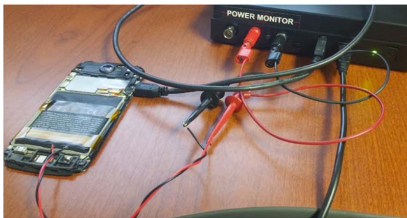
Figure 28 USB device connection, including main channel connection
