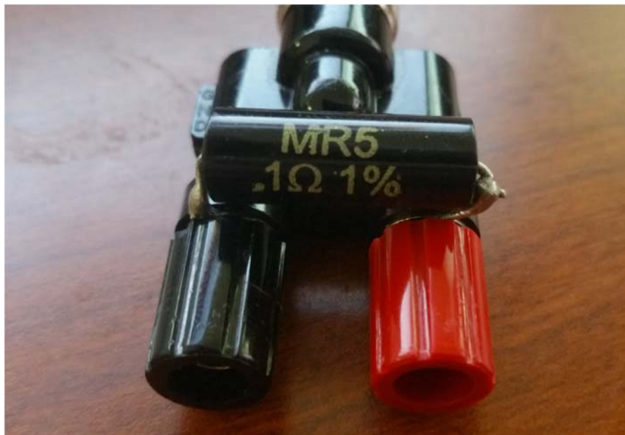
Figure 33 0.1 ohm sense resistor
