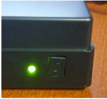
Figure 7 Front view: Engaged power button and powered-up green LED
