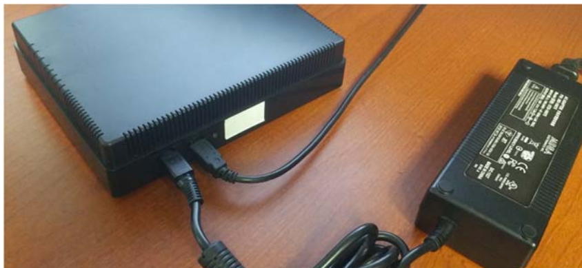
Figure 6 Back view: Power connector and USB connector
