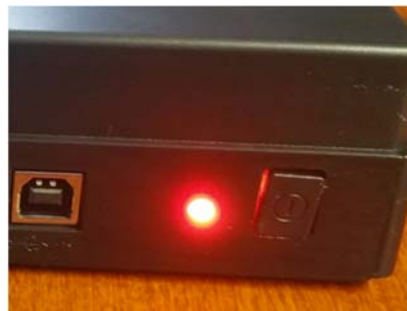
Figure 14 Amber LED indicator for over-current
